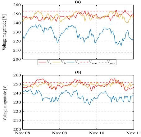
Voltage profile of the LV Lymbia feeder: current situation with 5% PV penetration b) near future operation with 30% PV penetration and 3 electric vehicles (from a KIOS study for EAC)
